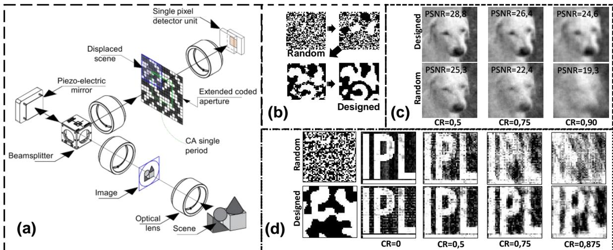
Fig. 1: Single pixel with a S-CA pattern. (a) Proposed architecture, (b) Illustrative pattern improvement, (c) reconstructed images for random and designed patterns varying the compression ratio (CR) and (d) experimental results for random and designed patterns varying CR.
