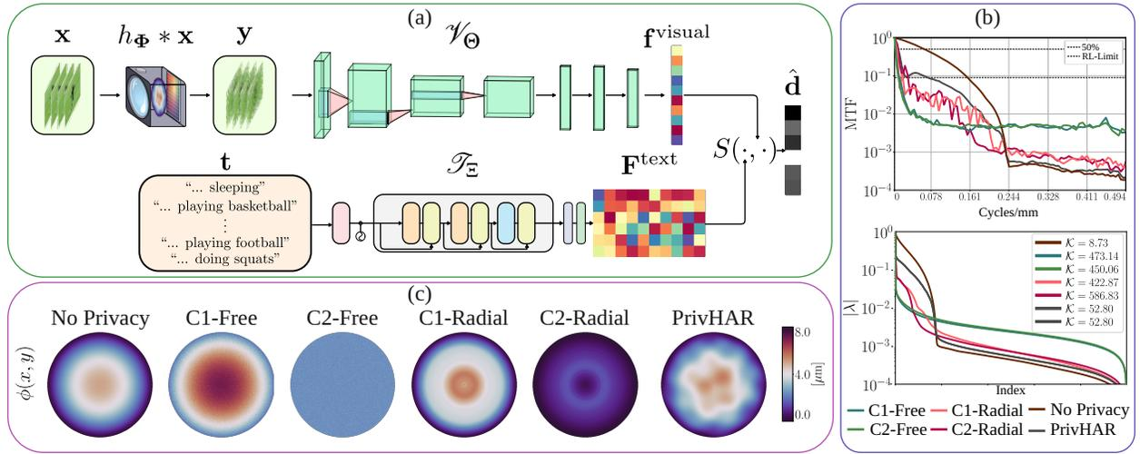
Fig. 1. (a) E2E scheme for privacy preserving multimodal action recognition, (b) MTF and eigenvalue distribution results, (c) Height map of the learned DOEs for different configurations.
