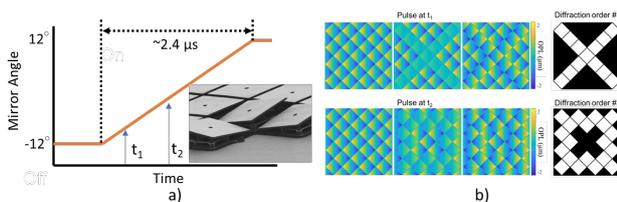
Fig. 1. Phase profile if DMD mirror array when (a) all the mirrors are actuated, (b) pattern is displayed, at timings  $t_1$  and  $t_2$  while mirrors are in motion [4].
