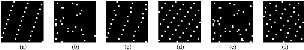
Fig. 1: CA of the 1<sup>st</sup> band: (a) 2 MUX  $\rho=0.56$ , CN= $3.98 \times 10^6$ , (b) Rand 2 MUX  $\rho=0.13$ , CN=2.49, (c) 2 MUX Rand  $\rho=0.27$ , CN=6.38, (d) 3 MUX  $\rho=0.36$ , CN= $1.32 \times 10^{12}$ , (e) Rand 3 MUX  $\rho=0.14$ , CN=3.84, (f) 3 MUX Rand  $\rho=0.26$ , CN=9.15
