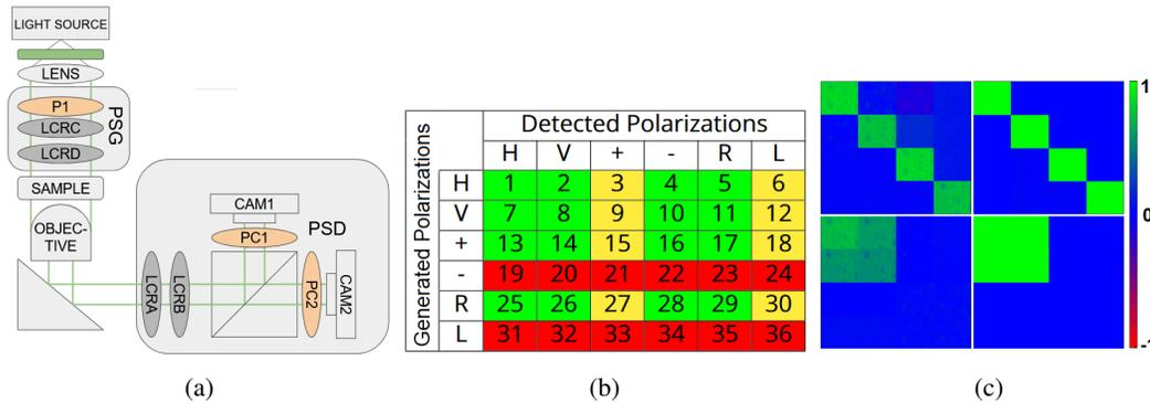
Fig. 1: (a) Proposed polarimetric system (b) SoPs used for MM calculations (c) Calibration results.
