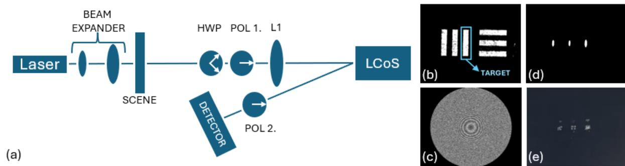
Fig. 1. a) Architecture b) Scene with target to detect c) DOE d) Simulated result e) Result.
