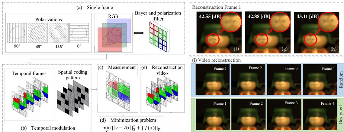
Fig. 1. Time polarized video compression's simulated system model.
