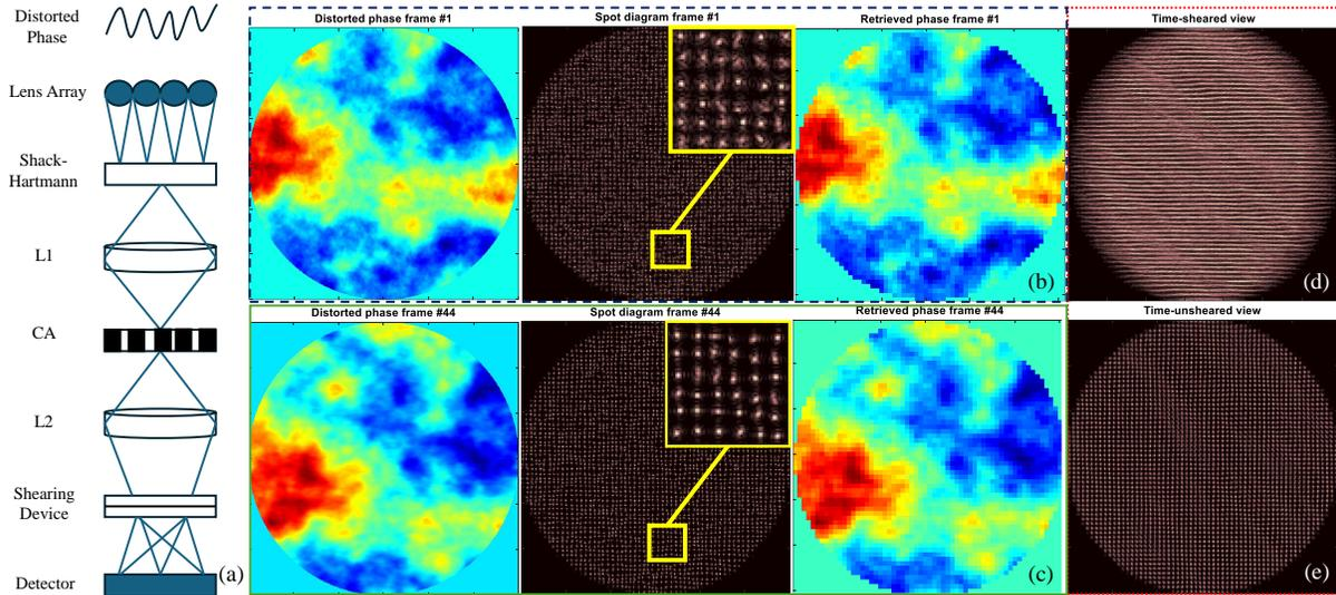
Fig. 1. (a) Proposed compressed optical Shack-Hartmann ultrafast photography system. (b) Frame #1 reconstruction process. (c) Frame #44 reconstruction process. (d) Spot diagram's time-sheared view. (e) Spot diagram's time-unsheared view.
