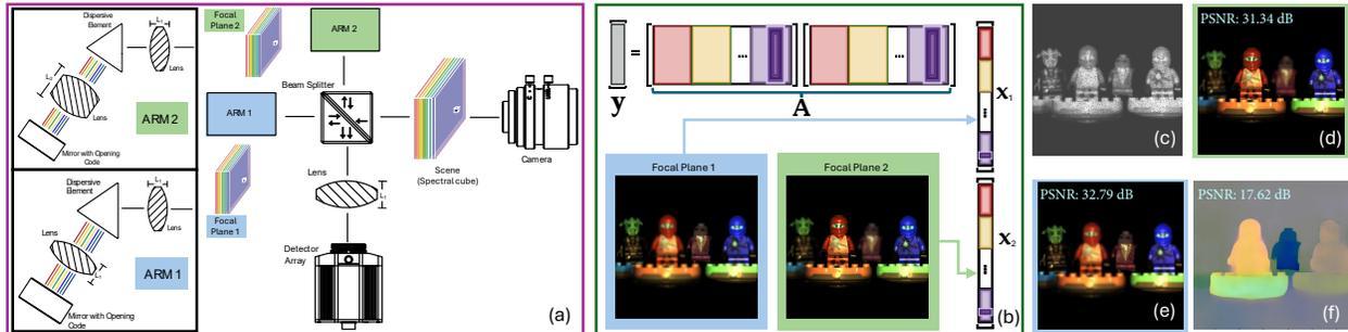
Figure 1. (a) Dual-arm DD-CASSI architecture. (b) Mathematical model. (c) Sum of encoded measurements from both focal planes received by the detector. (d) Recovered focal plane 1. (e) Recovered focal plane 2. (f) Depth estimation from the reconstructed focal planes.
