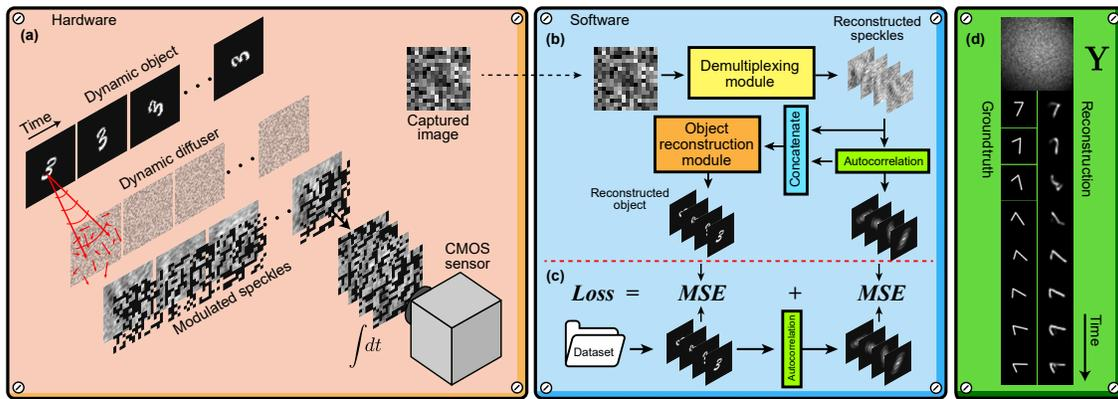
Fig. 1. The proposed compressive video scheme: (a) acquisition through scattering medium with a coded aperture, (b) The reconstruction model from speckles, (c) a loss function for optimization, and (d) experimental results comparing the reconstructed speckles measurements with the projected frames.
